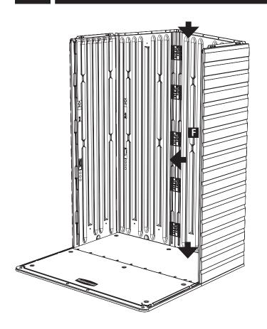
Using a screwdriver, punch out the screw holes on the top of **Right Back (F)** 4 places.
